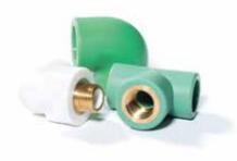
Engineered to withstand pressure under high temperatures, SABIC® PP-R have a very broad service temperature range, handling cold and hot water up to 70° C with a minimum service life of 50 years. It also delivers good performance under suitable pressure levels at temperatures reaching 90°C for periods under 50 years.
