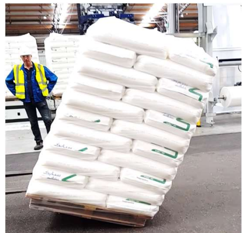
Tilt tests to check holding force use SABIC® solution
